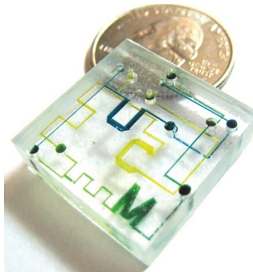
**Fig. 1** 3D Polystyrene microfluidics. Micromixer, demonstrating the blue (U) and yellow (C) channels on different layers mix on a 3rd layer to form the green M.
