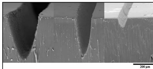
**Fig. 4** Different channel widths and heights. SEMs of channels demonstrating different channel shapes achievable using a simple scribing technique.
