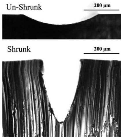
**Fig. 3** Before and after cross-sections of a channel. Note the shrinkage in width and corresponding increase in height.
