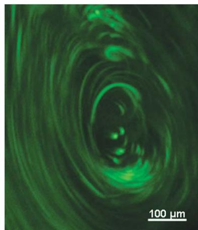
**Fig. 5** Microvortex (maximum intensity projection of 30 fps video) of fluorescent polystyrene bead streak-lines, representative of the vortices observed in the vias (see Fig 2) connecting the layers.
