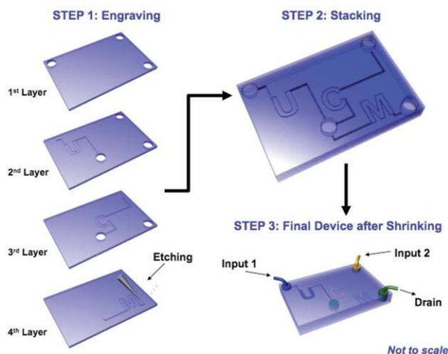
**Fig. 2** Process flow for 3D microfluidic chips. Each layer is scribed (using a syringe tip) and interconnect holes are punched. The layers are then aligned and placed in the oven for simultaneous shrinking and bonding.
